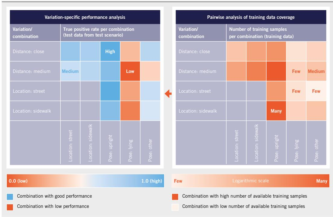
FIGURE 6 Variations-specific performance analysis based on data from the test scenario (left) and pairwise training data coverage analysis (right) (© Bosch)
